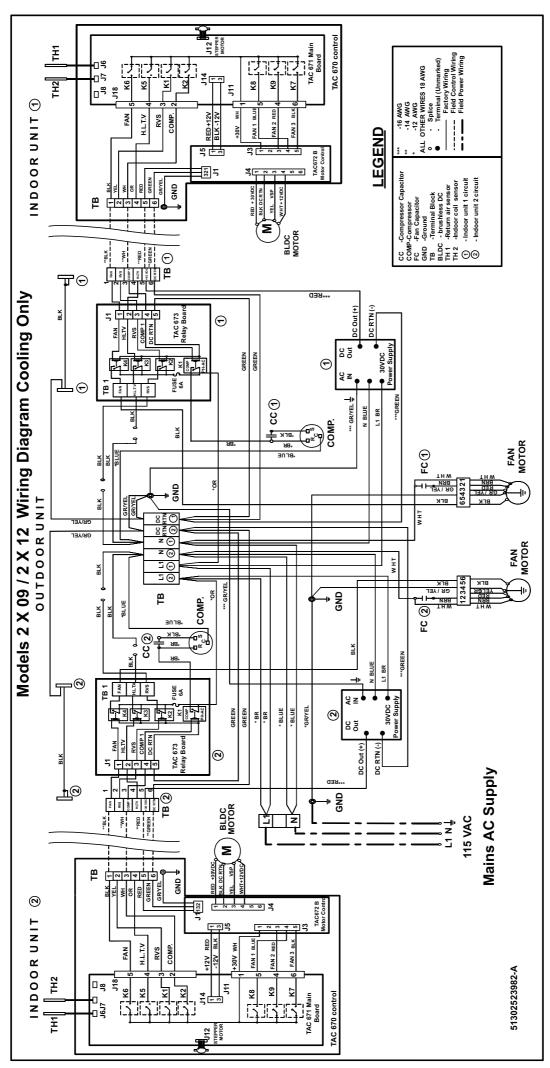
Fig. 14 System Wiring Schematic DFF2AH09J1A, DFF2AH12J1A FAN COIL WITH DFC2A318J2A, DFC2A318J2A Conden
